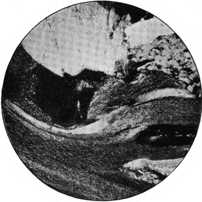
FIG. 1—THIN SECTION OF MASHED QUARTZ-PORPHYRY. AFTER FUTTERER.
